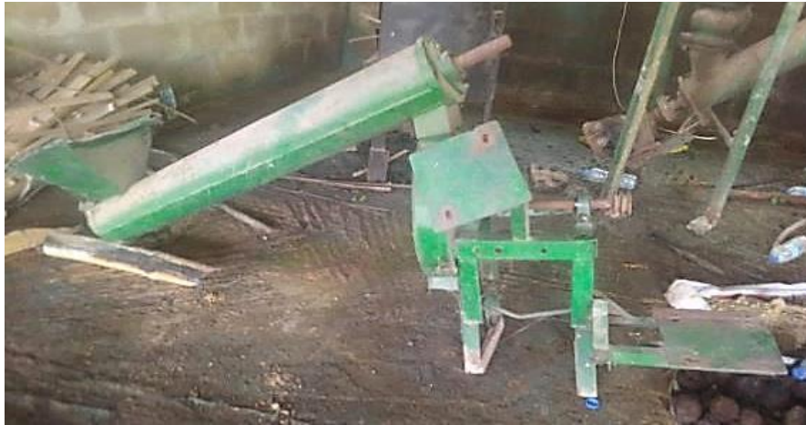
Figure 4: Fabricated Oil Palm Nut crack Machine and Conveyor
