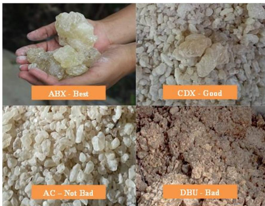
**Figure 3.** Quality Type of Resin Mat Cat Resin
